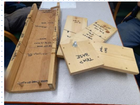
Cutting Templates and Jigs
